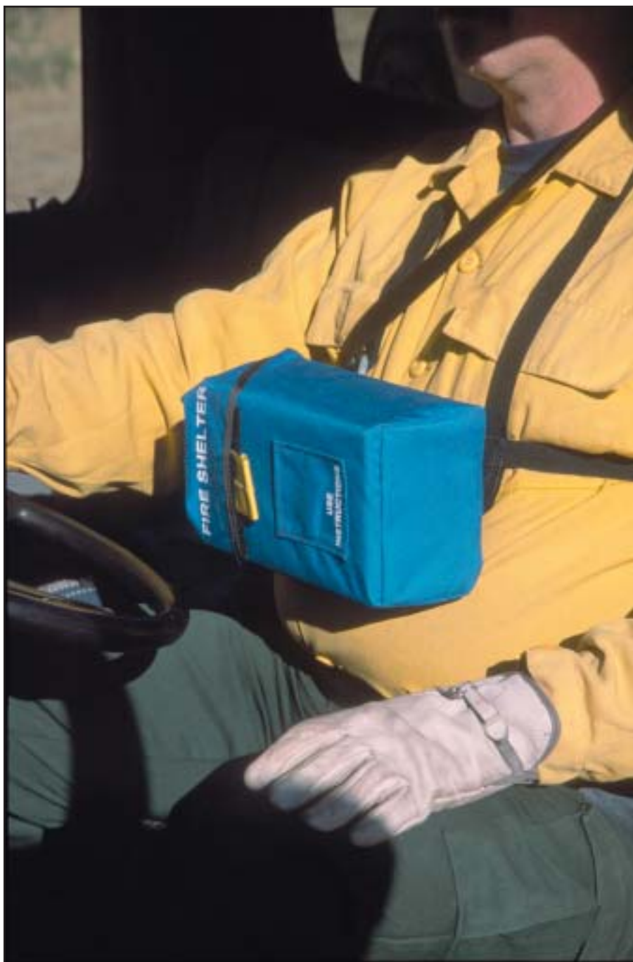
Figure 16—The chest harness is preferred by some operators of engines and heavy equipment.
