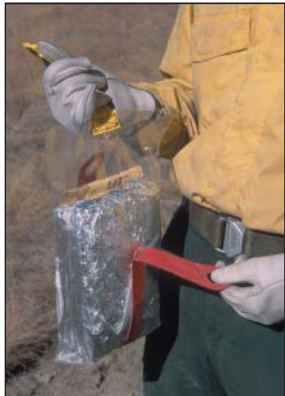
Figure 18—Pull either red ring to remove the plastic bag.
