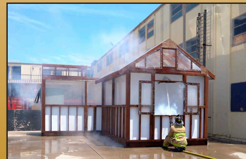
Proper - Nozzle movement stays fixed, minimizing air entrainment, and allowing window to self-exhaust
