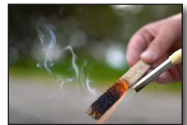
Figure 7-2 Solid fuel heated creating pyrolysis gases
