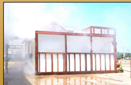
Both options create air entrainment. Pressurized smoke exits the opposite side ventilation opening
