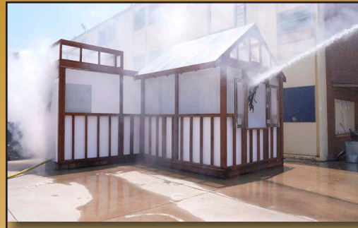
Minimal entrainment of air exits the window
