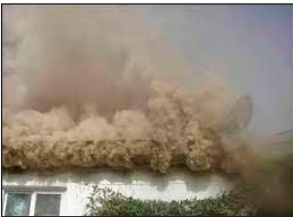
Figure 7-22 Reading Smoke - Location & Color - Indicating an attic fire with structural members
