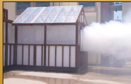
Maximum entrainment of air exiting the window
