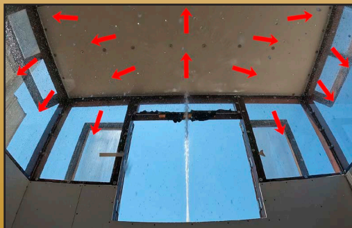
Proper - The steep angle allows the stream to make contact immediately, dispersing water along the entire compartment
