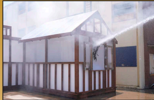
Opposite side ventilation opening shows no movement of smoke
