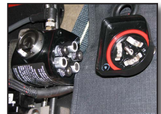
Figure 6-31 Air-Pak X3 Pro Battery Location, 6 AA’s
