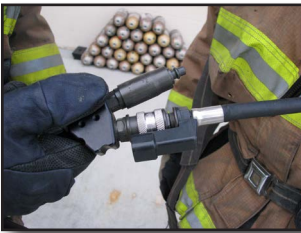
Figure 6-27 Alternative Buddy Breathing method - EBSS to Regulator (above 4 images)
