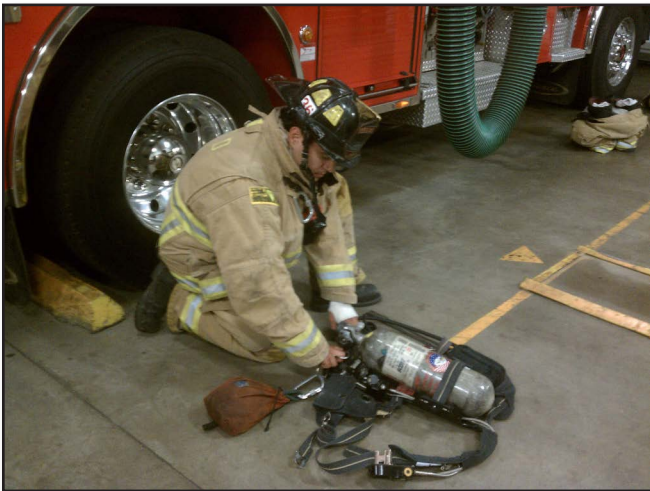
Figure 6-24 Bottle change with one firefighter
