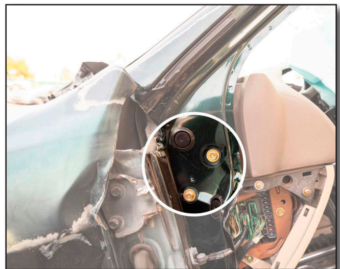
Figure 25-23 Locating the Transverse Beam
