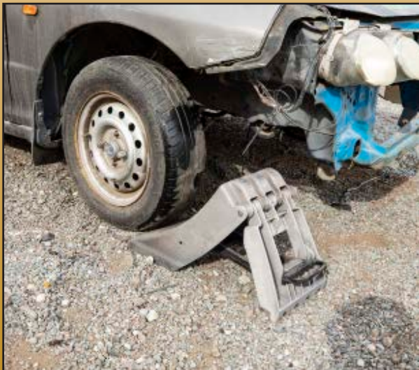
3. Stabilize wheels with cribbing or wheel chocks
