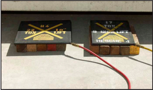
Figure 25-28 Side-By-Side Two Bag Lift
