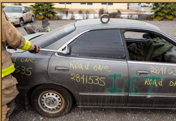
5. Strike the window at the lower corner with a hand tool
