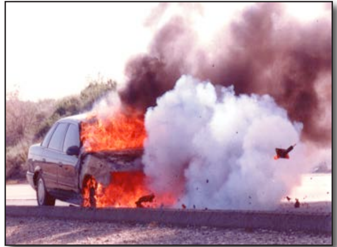
Figure 25-11 Bumper Strut Exploding
