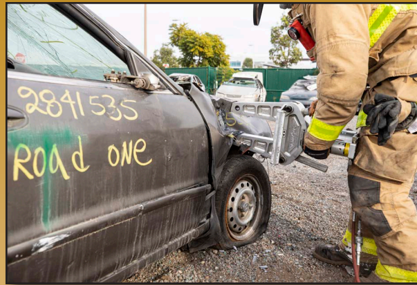
2. Clamp down the spreader tool to open up a purchase point at the door hinges
