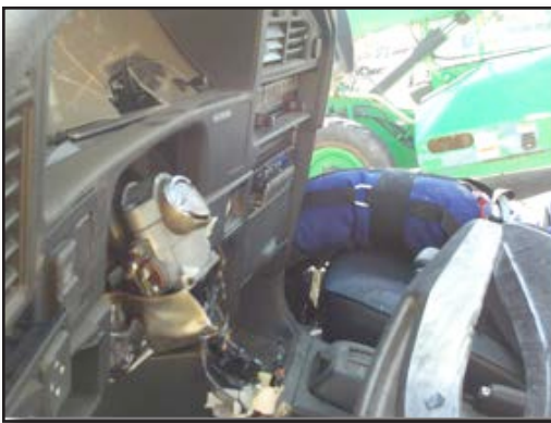
Figure 25-25 Complete Steering Wheel Removal
