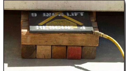
Figure 25-29 Solid Crib Bed for Achieving Maximum Airbag Lift
