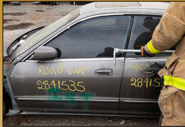
2. Strike the lower corner of the window with a hand tool
