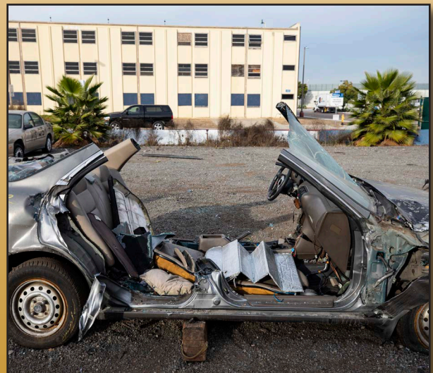
4. With enough personnel; lift and remove the roof off of the vehicle
