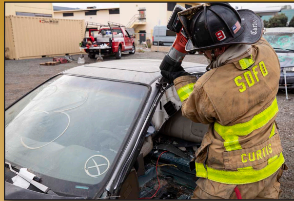
2. Make a relief cut towards the top A-Post
