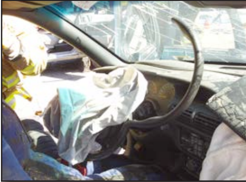
Figure 25-26 Cutting Steering Wheel
