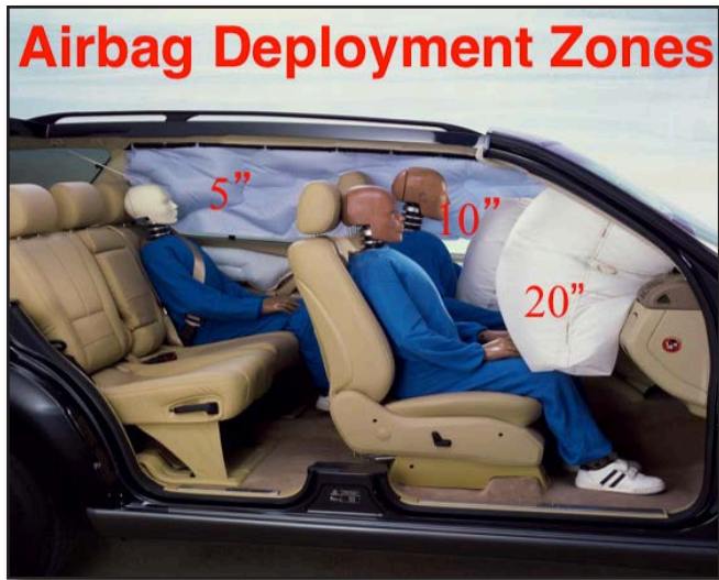
Figure 25-16 Airbag Deployment Zones “5-10-20” Rule
