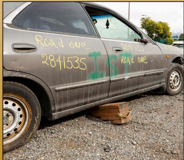
4. Place step chocks with anticipation of extrication needs
