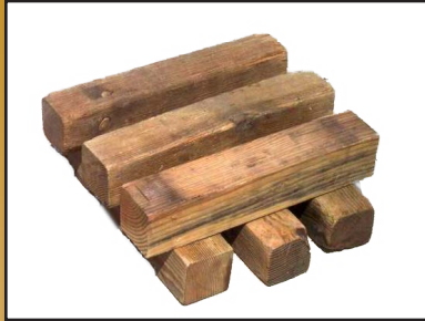
3 x 3 Crib Bed (Max 3:1 Height to Width)
