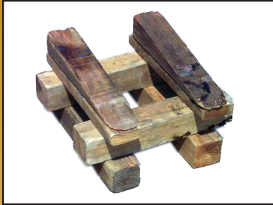
2 x 2 Crib Bed (Max 3:1 Height to Width)
