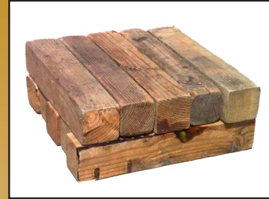
Solid Crib Bed (Max 3:1 Height to Width)
