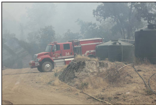
Figure 13-36 A good spot: facing out, not blocking the roadway, hoses in place, and clear of fuels
