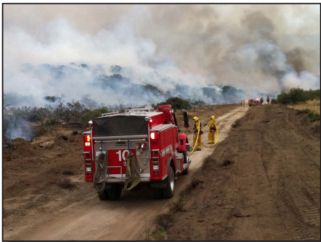
Figure 13-50 Back-Firing Operation - The pre-existing dirt road was used as the control line. Dozers widened the control line then crews set a back-fire using wind to their advantage. Brush crews were then spaced out along the control line to extinguish any spot fires that may have crossed the control line (right of road).
