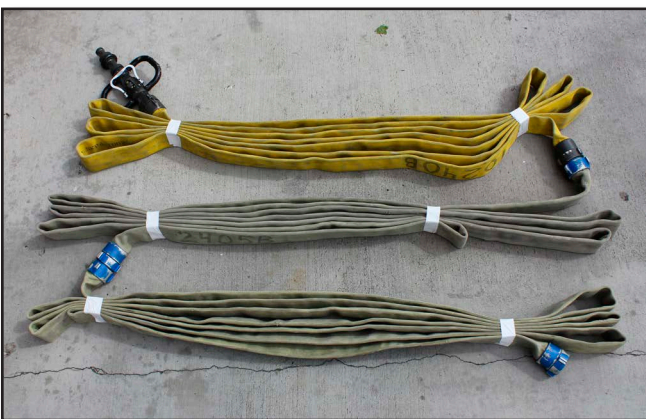
Figure 12-15 Fifty foot sections of 2 1/2" hose can be made into hose packs with duct tape. Once at the fire floor they can be connected easily, the tape can be removed, then quickly flaked out and deployed
