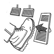
When you apply pressure to the throttle, the Jacobs Engine Brake is deactivated.
