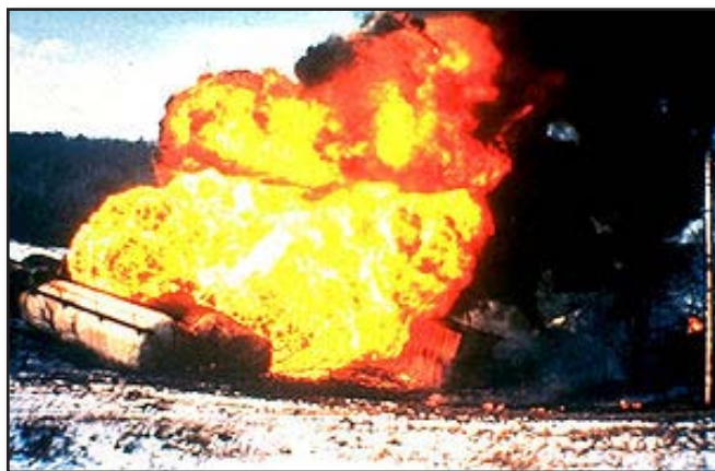
Figure 33-14 Boiling Liquid Expanding Vapor Explosion, aka, B.L.E.V.E.
