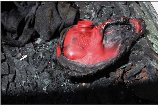
Figure 33-10 A gas can near the point of origin may indicate the use of an accelerant or an incendiary fire
