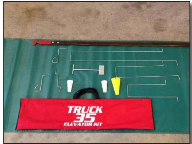
Figure 32-21 Standardized Elevator Rescue Kit found on all SDFD Truck Companies
