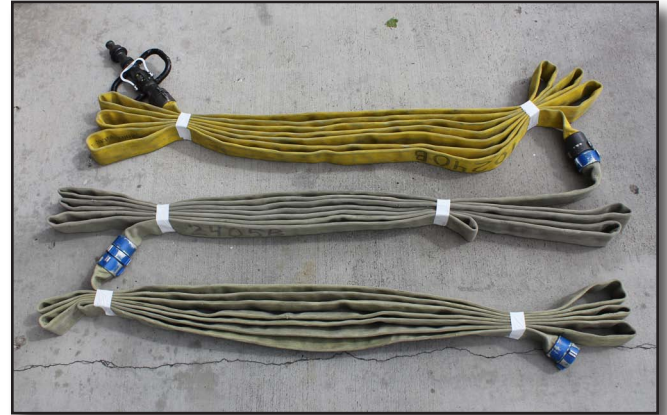
Figure 31-13 Fifty foot sections of 2 1/2” hose can be made into hose packs with duct tape. Once at the fire floor they can be connected easily, the tape can be removed, then quickly flaked out and deployed
