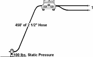
Step Two: Determine Available Pressure loss through each length
