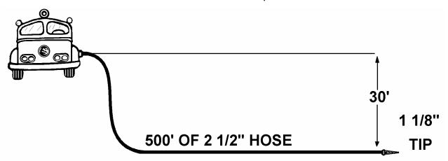
30  $(1.125)^2$  7 30 x 1.265 x 7 = 265.78 Round 265.78 to 270 Flow = **270** gpm
