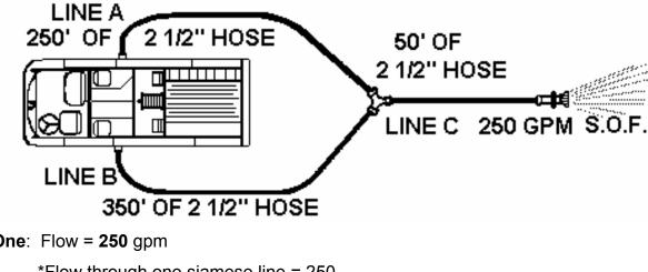
Step One: Flow = 250 gpm  $\geq$
