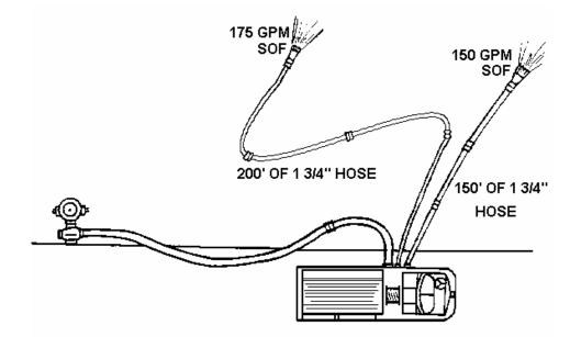
Step One: EF = Factor x gpm Flow (a) = 175 gpm EF (a) for 1 <sup>3</sup>/<sub>4</sub>" hose = 2 x 175 = 350 EF (a) = 350 gpm
