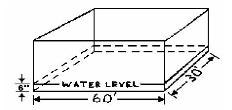
Weight = L x W x H x 62.5 Weight =  $60 \times 30 \times .5 \times 62.5$ Weight = 56,250 pounds Weight =  $\frac{56,250}{2000}$ Weight = **28 1/8** tons
