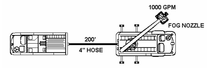
Step One: Flow = 1000 gpm EF = 1000 x .25 EF = 250 gpm
