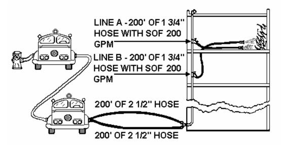
ALLOW 25 PSI LOSS FOR STANDPIPE SYSTEMS (SL) REGARDLESS OF SIZE. \* ALLOW 5 PSI GRAVITY LOSS (GL) PER FLOOR, ABOVE THE GROUND FLOOR, INCLUDING THE FLOOR THE NOZZLE IS ON. (DO NOT COUNT THE FIRST FLOOR. \*\*)
