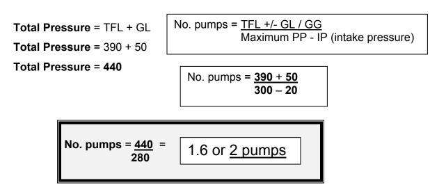
Using the above formulas, 2 pumps would be required for the relay to keep from pumping an excessive pressure.
