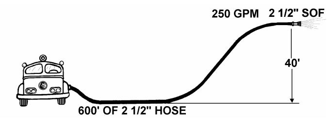
Step One: Flow = 250 gpm
