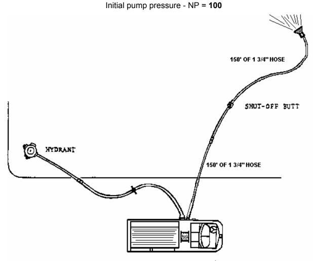
> Step One: Flow = 95 gpm
