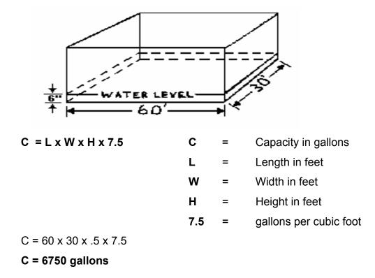
Example: Determine approximate capacity of rectangular tank 20' x 15' x 5'.
