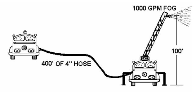
Step One: Flow = 1000 gpm EF = 1000 x .25 EF = 250 gpm
