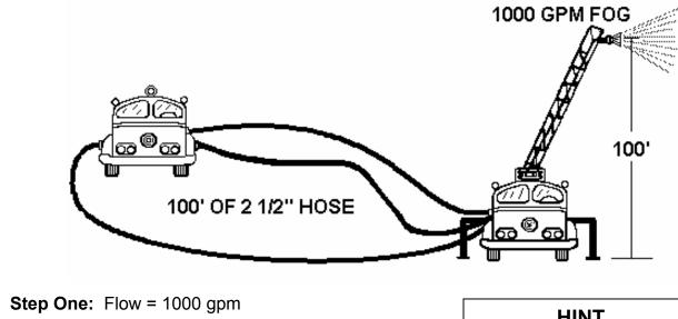
Flow through one line = 1000Flow through one line = 333 Round off single line flow to 330 Flow = **330** gpm
