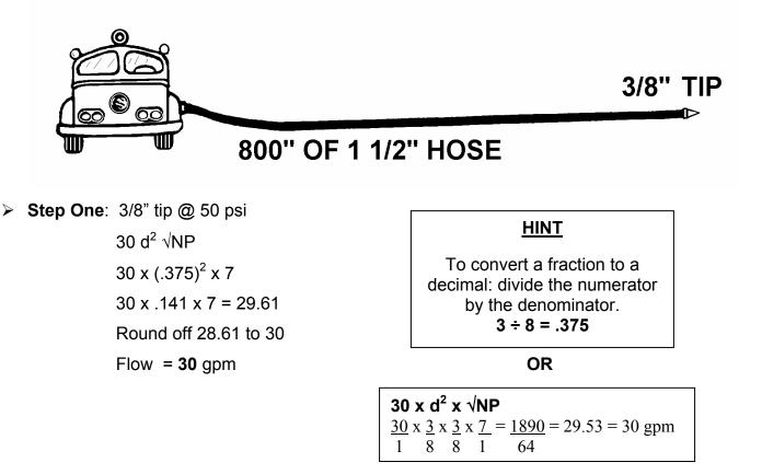
\*EF = Factor x gpm EF for 1 ½" hose = 3.6 x 30 = 108 EF = **110** gpm
