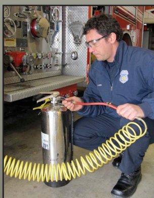
Charge extinguisher with compressed air
