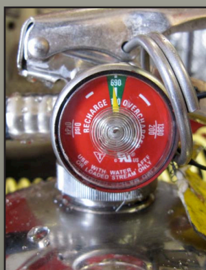
Ensure the air pressure gauge is in the green
