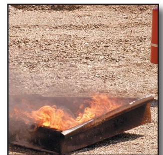
Figure 10-8 Steel pan used for Class B fire rating test
