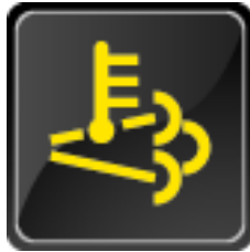
High Exhaust System Temperature (HEST)
