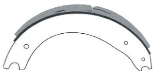
Cracks or voids that exceed 1/16 inch in width. Cracks that exceed 1 1/2 inches in length.
