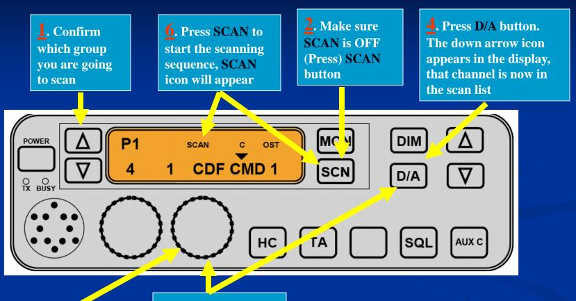
3. Rotate channel SELECTOR knob to the channel you want to add to scan
