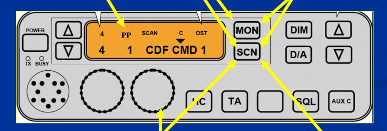
1. The Priority 1 channel is by default the channel you have selected in the display before pressing the scan button. In other words, when you want a specific channel to be priority, rotate the channel selector to that channel and stop, press [SCN]. This channel is now your Priority 1 channel.
