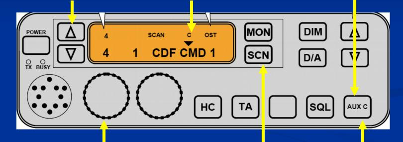
2. Use the channel select knob to dial up the desired channel to add to the command group from any group in the radio.
