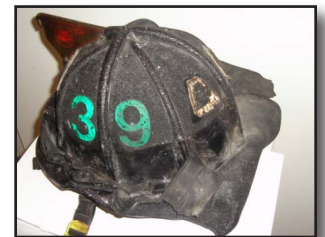
Figure 3-16 Helmet Failure Due to Heat
