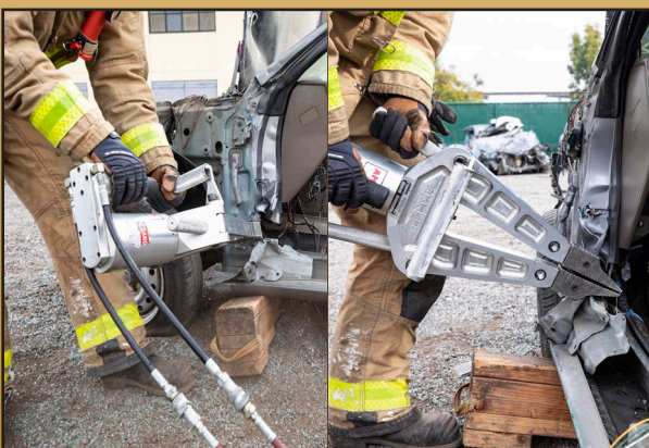
5. With the spreaders, pinch the metal material between the two relief cuts and bend it outwards. Next, place the spread tool in the created space at a slight downward angle
