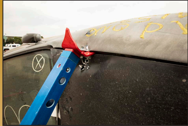
2. Place strut against the vehicle with the desired angle (45 Degrees)
