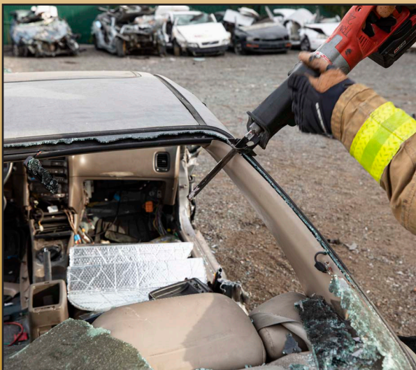
3. Cut all surrounding posts using either a sawzall or hydraulic cutter
