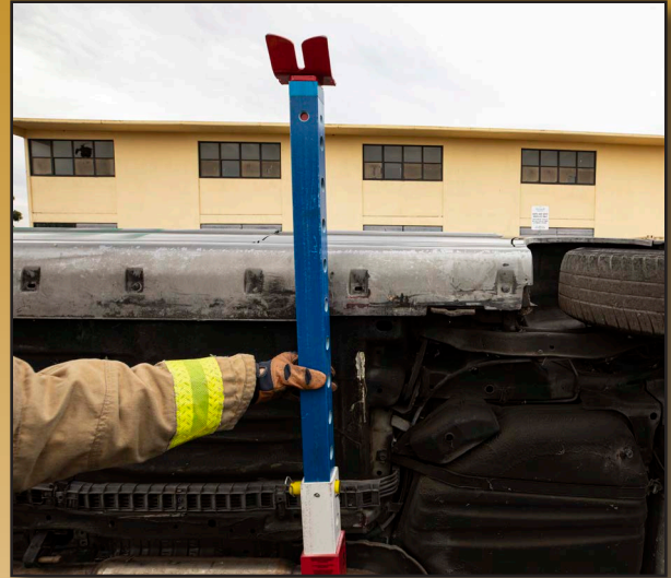
2. Extend Strut 16" above your insertion point
