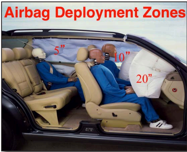
Figure 25-16 Airbag Deployment Zones “5-10-20” Rule
