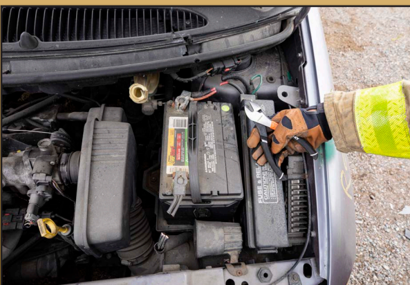
5. Next place a chunk cut on the positive terminal
