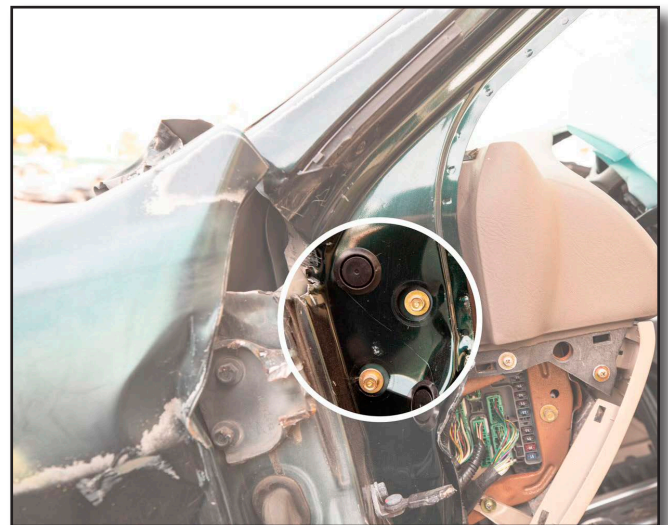
Figure 25-23 Locating the Transverse Beam
