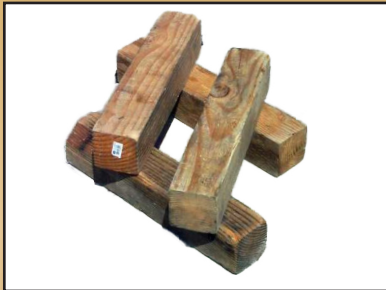
Parrallelogram Crib Bed (Max 1:1 Height to Width)
