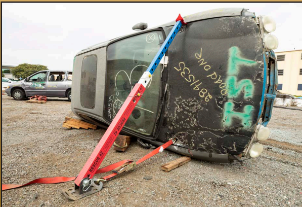
4. Single tension buttress is placed at the roof side engine compartment
