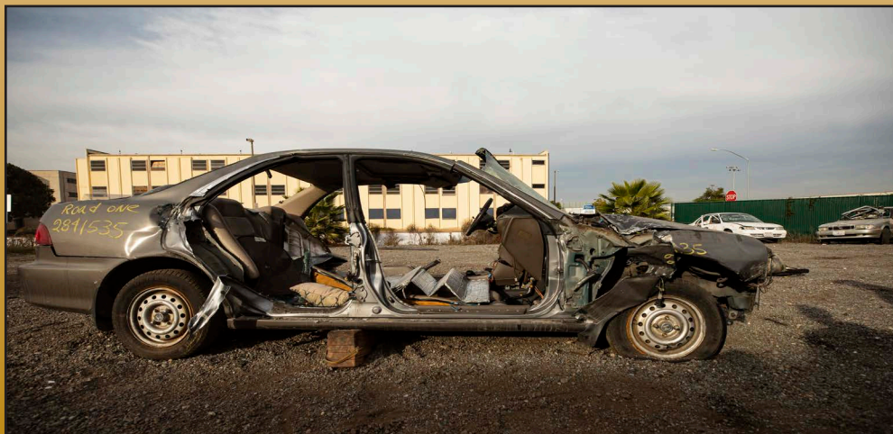
5. Door is taken off for a complete door removal
