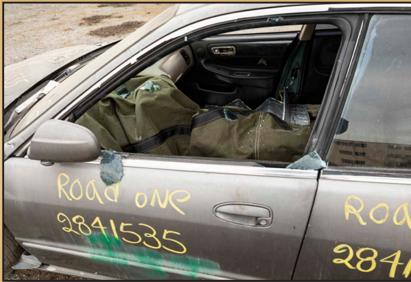
3. Strike the window and remove any remaining glass
