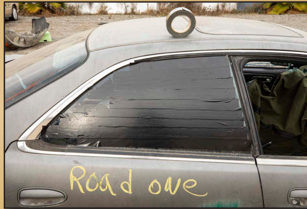
4. An alternative method is to place duct tape on the intended window
