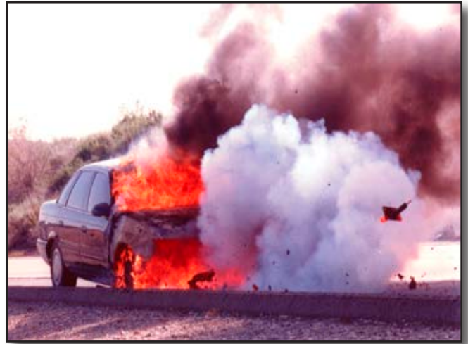
Figure 25-11 Bumper Strut Exploding
