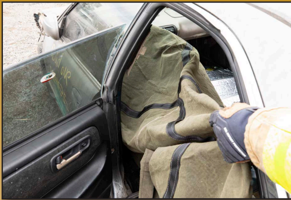
1. When taking glass near a victim, take precautions to cover and protect the victim
