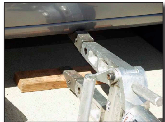
Figure 25-27 2 x 2 Crib Bed (top) and Lifting with the Amkus Spreaders (bottom)
