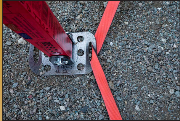
2. Strap is ran through the struts base plate
