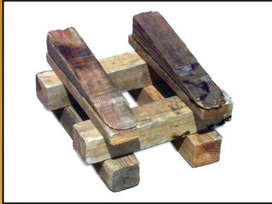
2 x 2 Crib Bed (Max 3:1 Height to Width)
