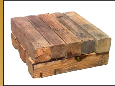
Solid Crib Bed (Max 3:1 Height to Width)
