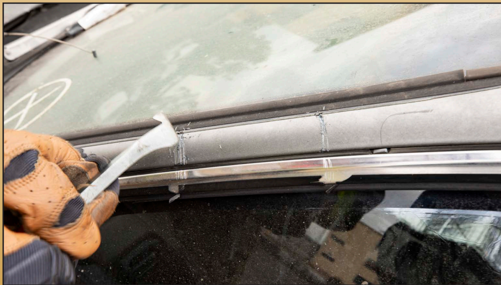
3. When cylinders have been located, mark the location on the exterior of the vehicle for all personnel to see
