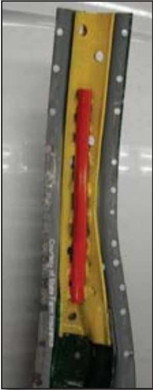
Figure 25-8 “B” post reinforcement bar (red)
