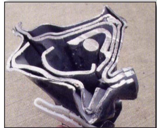
Figure 25-6 Multiple layers of a “B” post with a reinforcement bar (above two images)
