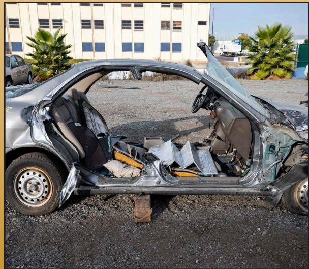
4. With the B-Post now removed, a complete side wall removal is completed
