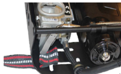
Figure 3.15-4: Waist to Shoulder Strap Install Step # 3
