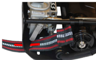
Figure 3.15-3: Waist to Shoulder Strap Install Step # 2
