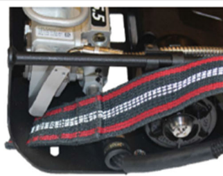
Figure 3.15-2: Waist to Shoulder Strap Install Step # 1
