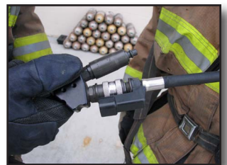
Figure 6-28 Alternative Buddy Breathing method - EBSS to Regulator (above 4 images)
