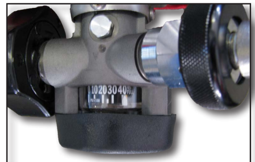
Figure 6-7 Cylinder Valve Assembly w/o Hansen Valve
