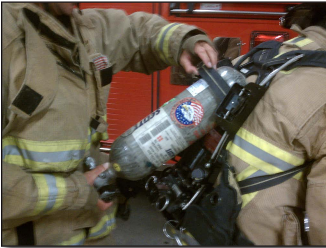
Figure 6-26 Bottle change with two firefighters
