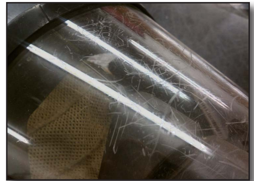
Figure 6-31 Scratched Face Piece
