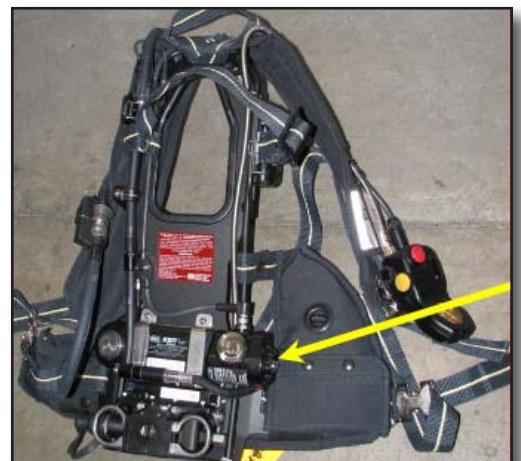
Figure 6-3 NxG7 Battery Location (6 AA)
