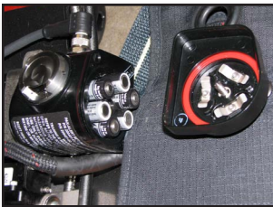
Figure 6-33 NxG7 Battery Location, 5 AA's
