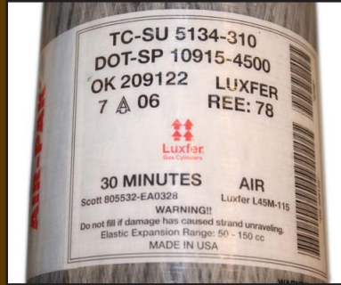
DOT #, Date of Manufacture, and Initial Hydro Test Date
