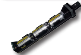
Figure 6-32 NxG2 Battery Location, 3 C's
