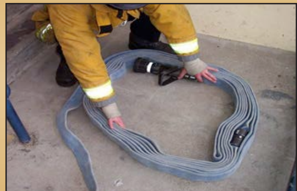
Spread open the hose pack, but do not flake out hose until charged.
