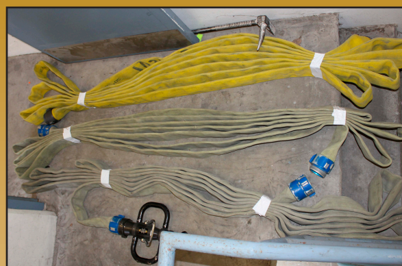
Lay out the hose packs on the fire floor landing aligning the couplings & attach nozzle
