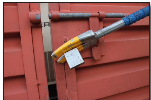
Figure 21-29 Twist or shear lock with claw of halligan bar to break or open
