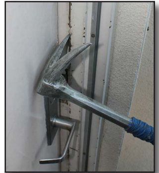
Figure 21-9 Alternate Option - GAP/FORCE the door with the Adz
