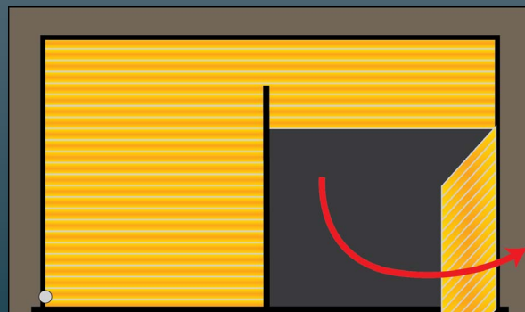
Swing the cut door open, hinging on the track
