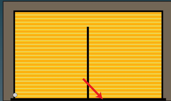
Cut a diagonal relief cut to allow the rescue saw to fit into the doorway to cut the angle iron on the bottom
