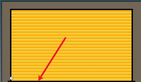
Cut #1 is made downward from the center of the door at a 60 degree angle
