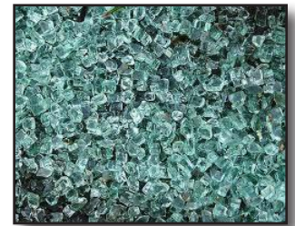
Figure 21-52 Broken Tempered Glass
