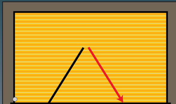
Cut #2 is made downward from the center of the door at a 60 degree angle in opposite direction. Do not cross your cuts
