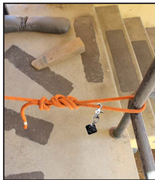
Figure 18-3 Utility rope can be used as a tag line when anchored outside (L). Knots can also be tied in a tag line as reference points for other firefighters (R).
