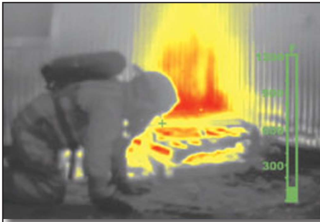
Figure 18-5 View of a fire through a TIC (L). View of smoke through normal vision (Top R), same view using a TIC (Bottom R).
