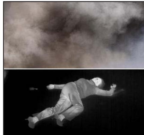
Figure 18-5 View of a fire through a TIC (L). View of smoke through normal vision (Top R), same view using a TIC (Bottom R).
