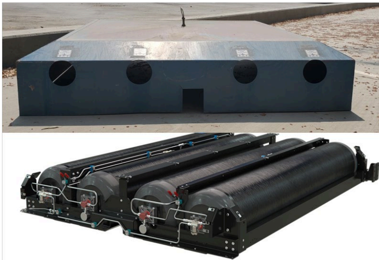
View of typical roof-mounted cylinder configuration and cylinder cover from similar Trash Truck. Cylinder cover size is 78"L x 85"W and approximately 200lbs. Single cylinder size is 77"L x 16" diameter and 153lbs.
